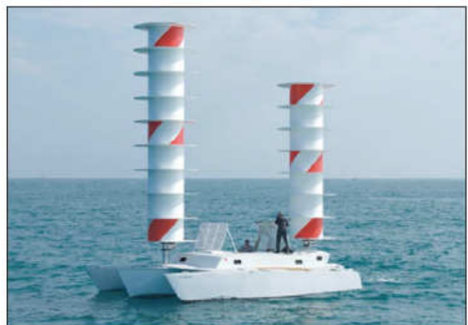
Figure 1. Wind-driven spray vessels for enhancing cloud albedo to reduce global warming. Left: an artist's impression of such a vessel. Right: Cloudia, an existing vessel working on the same principle. Both pictures taken from [4], copyright J MacNeill and Discovery Channel, respectively.
