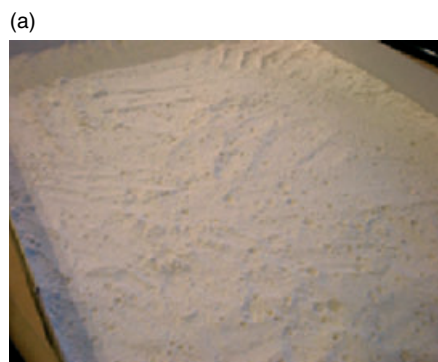
Figure 1. A platform covered by flour: (a) after a rainfall event with many raindrop hits; (b) the raindrops adopt a spherical shape when hitting the flour.
