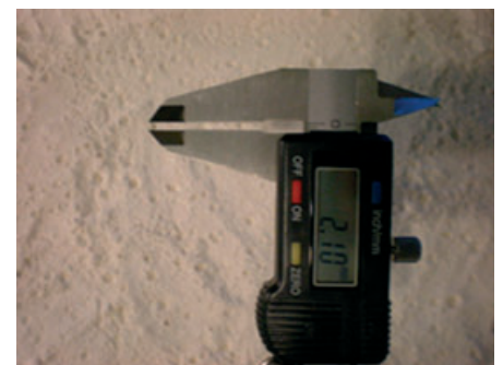
Figure 2. Measuring a raindrop on the flour-covered platform using an electronic sliding caliper.
