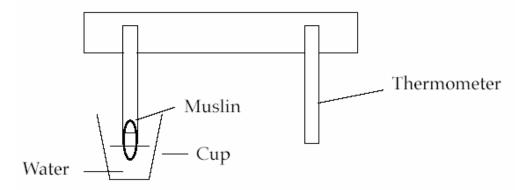
Put the prism on a stack of textbooks so that one of the thermometers can be placed inside the upper part of a cup. Half-fill the cup with water and position it beneath one of the thermometers. Wrap the muslin around the bulb of the thermometer and have the rest dangling in the water. After 10 minutes, take the readings of both thermometers and use this table to work out the relative humidity.
