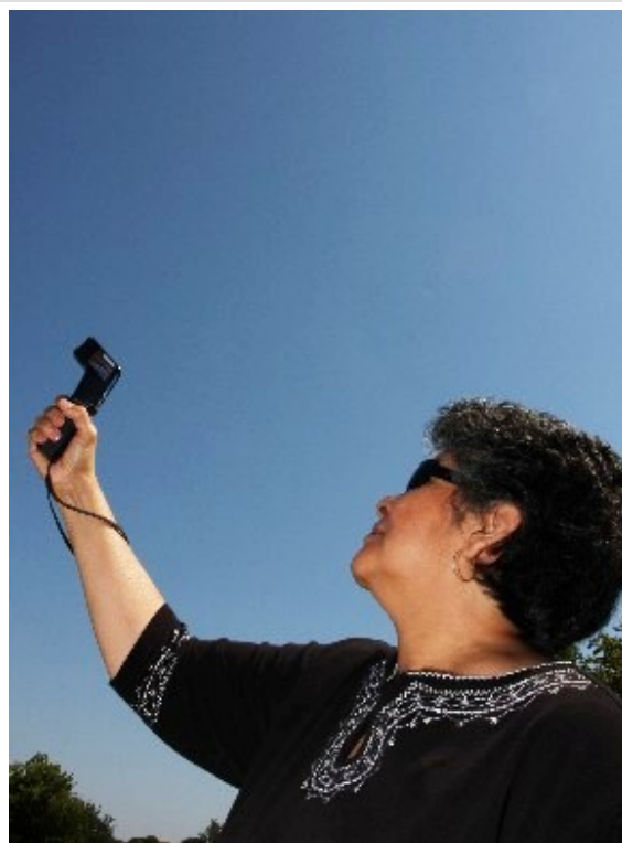
Measuring the temperature of the sky (27 F or -3 C). Image courtesy of Forrest M. Mims III
