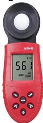
Fieldwork investigations are sometimes connected with other aspects of the environment such as plant growth, forest density, etc, for which light levels are also required. These can be measured with a simple hand-held light meter such as the one illustrated. USB dataloggers are also available to record light levels.
