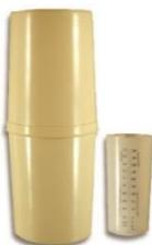
Rainfall is easy to measure using simple, cheap manual rain gauges such as that shown above. The rainfall amount should be recorded at the same time each day, and then emptied. To avoid the gauge being blown over by the wind, it should either be placed in a slight hole in the ground, or partially buried in a flower pot or similar.
