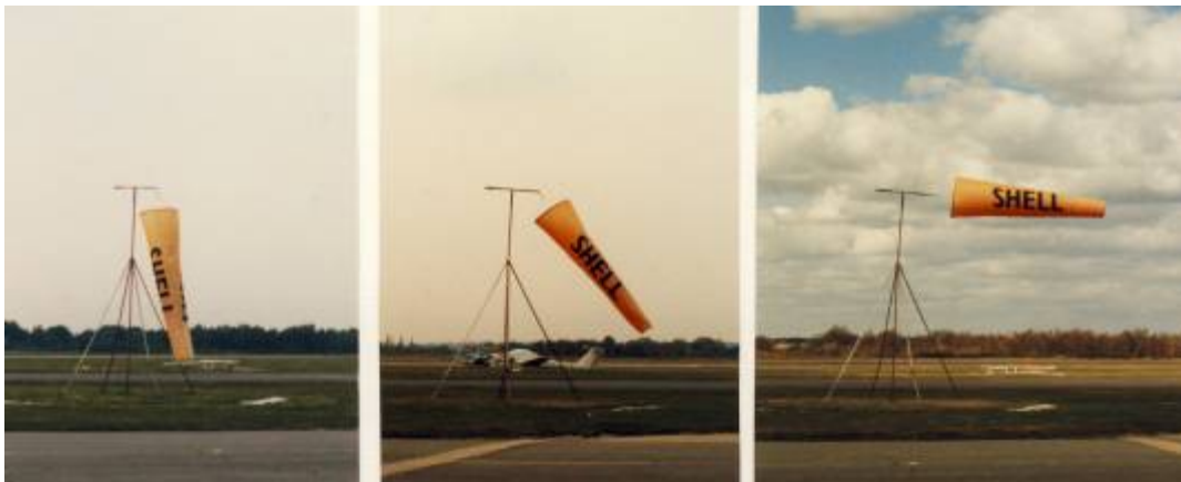
Figure 20. A wind sock on an airfield shows pilots wind strength and direction
