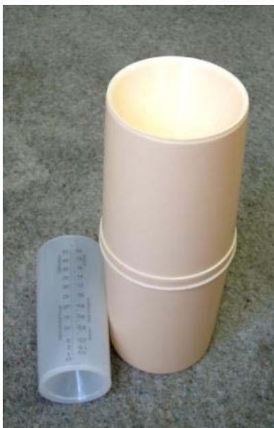
Figure 13. A relatively cheap plastic rain gauge with funnel and measuring cylinder (which goes inside the rain gauge when in use)
