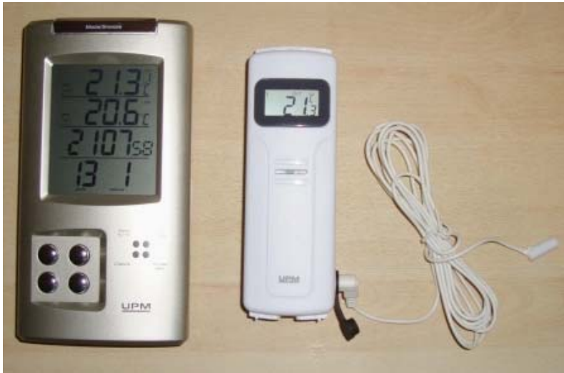
Figure 12: Outside measurements of temperature and RH, from sensors at the end of a wire, are sent by the transmitter (white, right) to the indoor receiver and display unit (silver, left).
