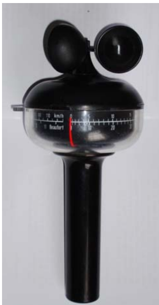
Fig 18: A mechanical cup anemometer, showing the scale and red pointer.
