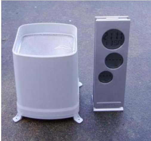
Figure 14. A tipping-bucket wireless rain gauge, with display which goes indoors.
