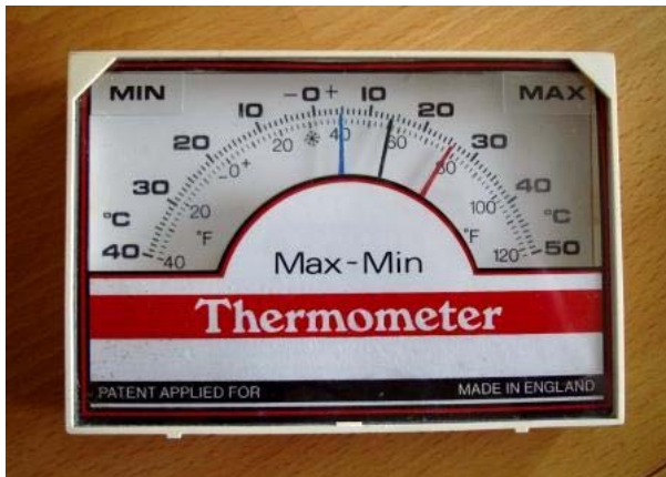
Figure 4: An easy-to-read maximum-minimum bimetallic thermometer. The air temperature (black pointer) is about 14C, the minimum (blue) since last reset is 5C and the maximum (red) is 26C.
