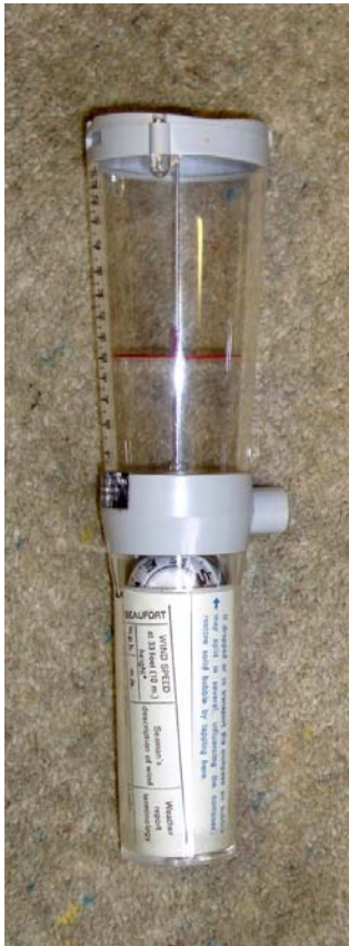
Figure 17: A ventimeter for measuring windspeed and (with the compass in the handle) wind direction.
