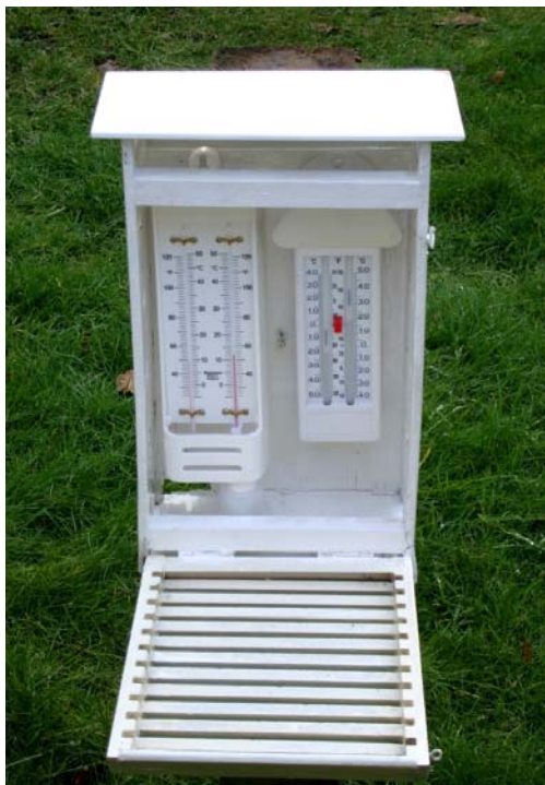
Figure 7 A simple louvered thermometer screen (available as a kit or ready built) with maximum-minimum and wet and dry bulb thermometers inside, mounted on a post in a garden lawn.
