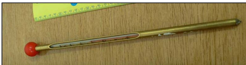
Figure 8: A soil thermometer, which is pushed into the ground so that the bulb is at a depth of 20cm.
