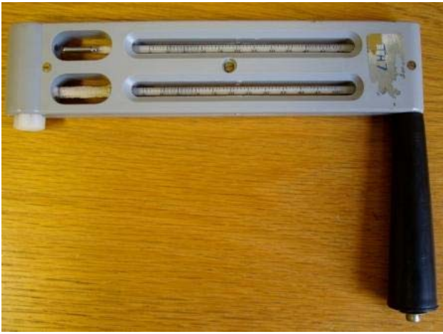
Figure 10. This type of wet- and dry- bulb thermometer is known as a whirling psychrometer
