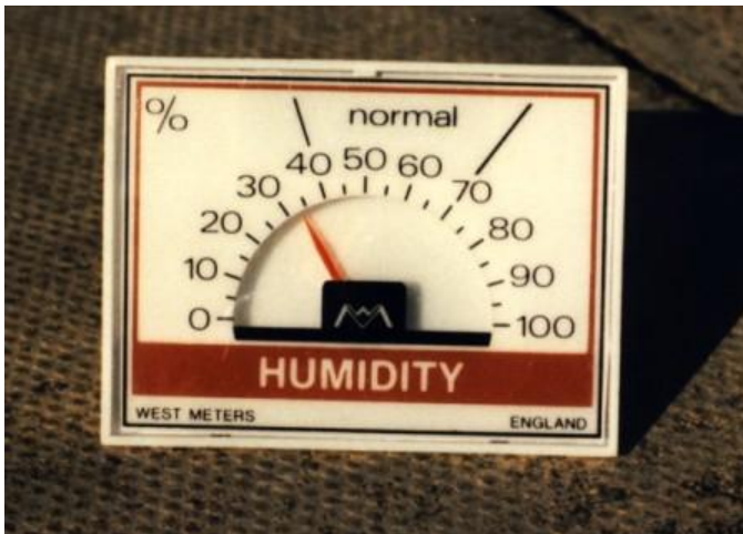
Figure 11: Simple and cheap paper hygrometer, reading RH directly in percent.
