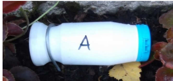
The USB temperature logger (left) and protected by a yogurt pot (right) and pinned down
