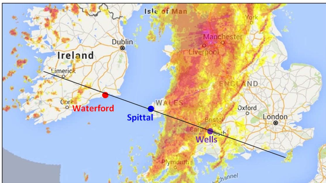
*The radar rainfall map with the initial station (Wells), the line drawn through it roughly at right angles to the front, and the two other stations near the line at which good cold front temperature drops can be seen on their WOW graphs.*
