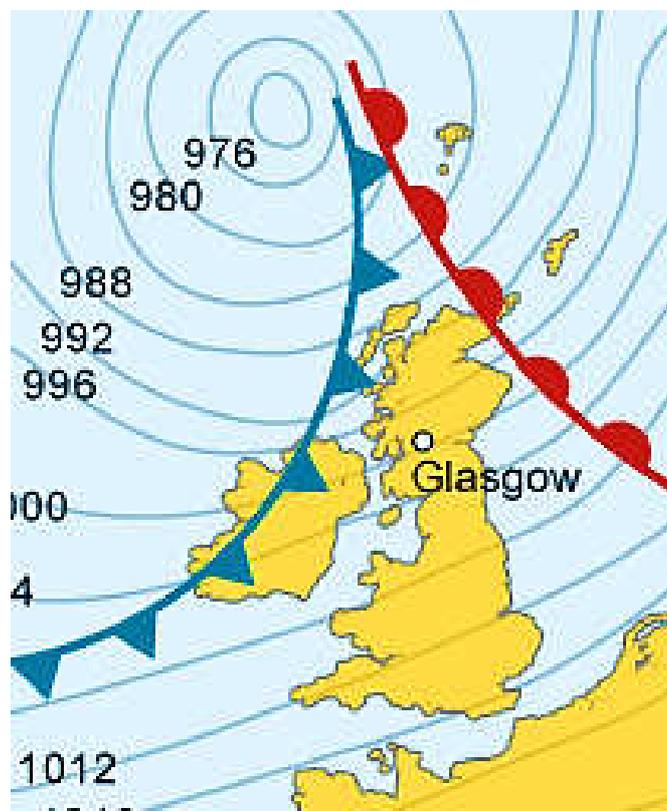
*A typical mid-latitude weather system, with a depression to the north-west of Scotland. The cold front is thick blue line with triangles showing the direction of travel; warm front is red line with semicircles. Pale blue lines are isobars with pressure in hPa (or millibars) written on them.*
